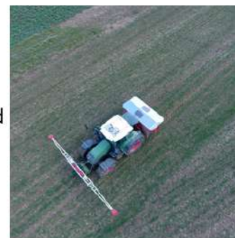
Tractor with nitrogen sensor and fertiliser spreader. A plant sensor mounted at the front of the tractor measures the wheat's nitrogen requirements and adjusts the fertiliser application rate by the spreader mounted at the rear of the tractor.
